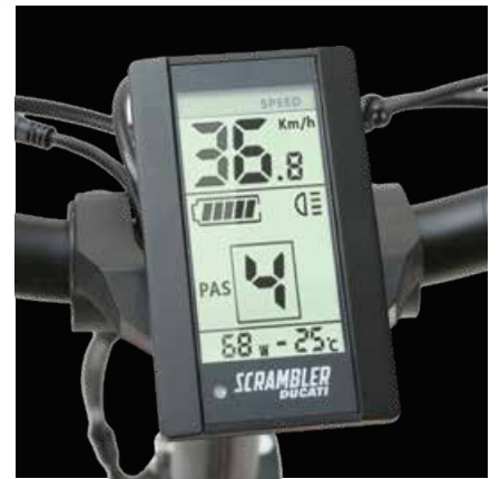
Display with twilight and temperature sensor
